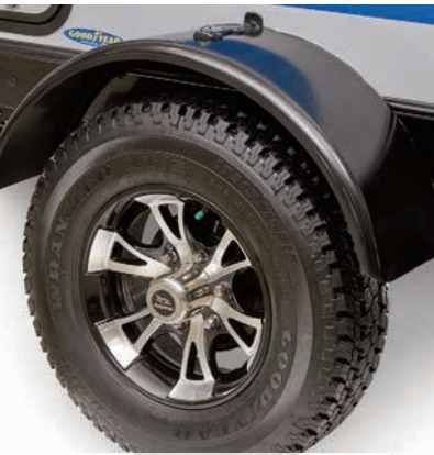
GOODYEAR® TIRES WITH DEXTER® TORSION AXLES AND SELF ADJUSTING BRAKES
